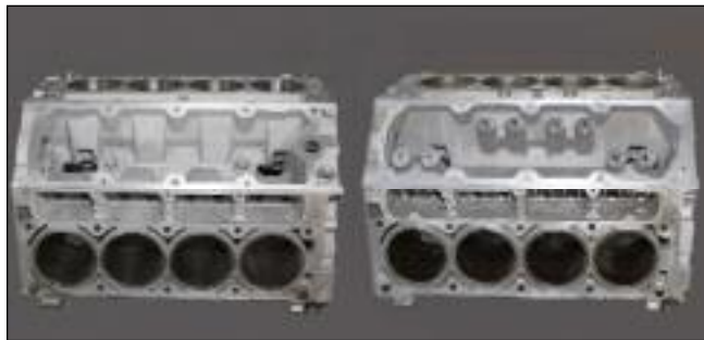
The Gen IV blocks have 8 oil ports in the valley for AFM instead of the two knock sensors that were located in the valley on the Gen III motors.
