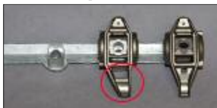
The intake rockers had to be offset by 6.0mm to clear the large, rectangular ports on the 823/ 5364 heads that were installed on the 6.0L Gen IV engines beginning in '07.
