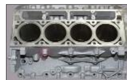
The Gen IV aluminum blocks have one extra bolt hole on the passenger side.
