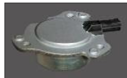
The VVT motors have an electric solenoid that modulates the oil to the phaser so it can advance or retard the cam.
