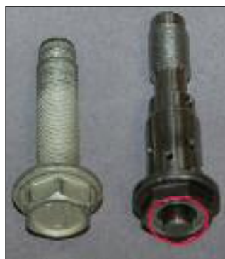
The cam gear was held on with one big bolt beginning in '07. If the engine had VVT, the bolt had an actuator valve in the center.
