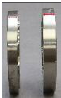
The oil pump for the aluminum engines with AFM and/or VVT had 33% more volume. Note the difference in the width of the gerotor on the right.
