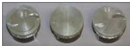
Most of the 6.0L Gen IV engines came with either flat top or dished pistons that had valve reliefs for VVT, but the ones for the LS2 didn't have reliefs because it didn't have VVT.
