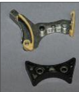
The Gen IV motors came with the chain guide in '05 and '06, but they all got the blade-style tensioner beginning in '07.
