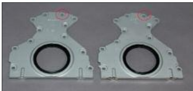
There's one bolt hole on the rear cover for the FWD (right) that's relieved to clear the smaller Buick bell housing.
