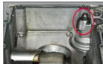
The shield that fits over the AFM relief valve in the pan deflects the oil down and away from the crank so it doesn't end up on the walls.
