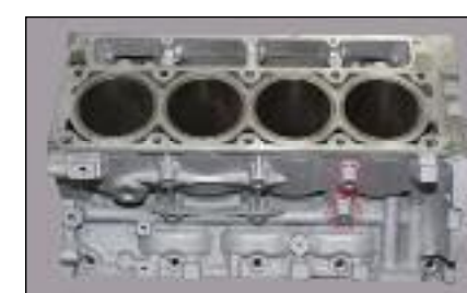
The Gen IV aluminum blocks have two extra bolt holes on the driver's side.
