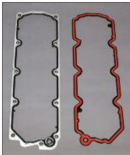
The perimeter gasket on the left is used for the cover without AFM and the one on the right is used for the one with AFM.
