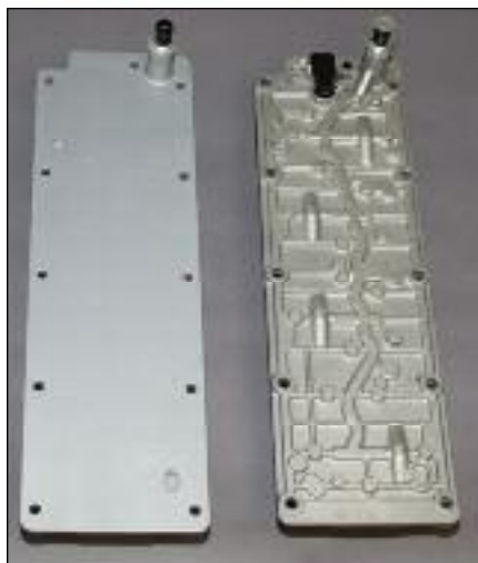
The Gen IV engines without AFM had a flat cover (left) that sealed off the valley and the oil ports. The lifter oil management assembly (right) was used on the engines with AFM.
