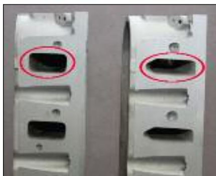
The 6.0L Gen IV motors got the 823/5364 castings with the big rectangular intake ports instead of the ones with the smaller cathedral ports that were used on all the rest of the Gen IV engines.
