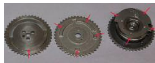
The three bolt gear with a 1X sensor was replaced by the 1 bolt gear or phaser that had a 4X sensor in '07.
