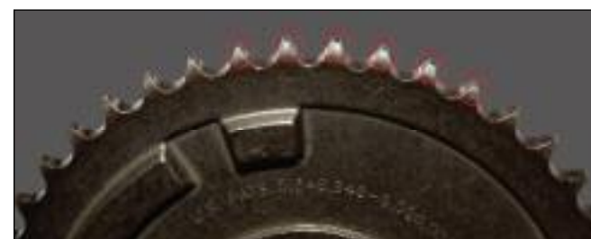
Note the difference in the shape of the teeth on the cam gear. This asymmetrical design reduces chain noise.
