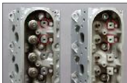
The rectangular port heads (left) have round bolt pads instead of the square ones, so there are two different rocker supports.
